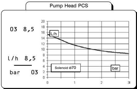
Flow rate indicated is for H<sub>2</sub>O at 20 °C at the rated pressure. Dosing accuracy ± 2% at constant pressure ± 0,5 bar.
